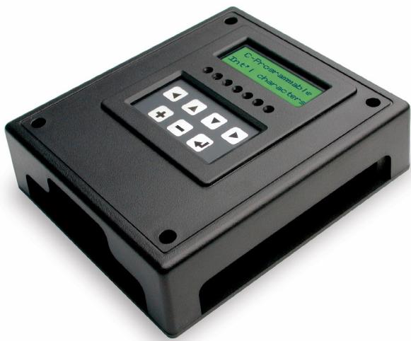
A 7-key, 122 x 32 graphic display is available as a cost-effective user interface. A panel-mount, water-resistant NEMA 4 version is also available. Keypad legends are easily modified using customizing printed paper inserts. User-programmable LEDs provide quick-status feedback. The entire board/display/keypad assembly mounts in an integrated plastic enclosure.
